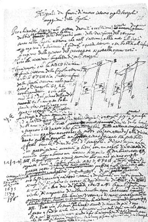
Fig. 3. Viviani sketches for Santa Maria del Fiore ties calculation
