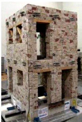
Fig. 13. Masonry model, reinforced using injections, on the shaking table
