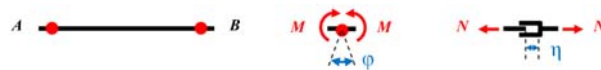
Fig. 2 Schematic representation of a beam finite element with plastic joints (at edges A and B )
