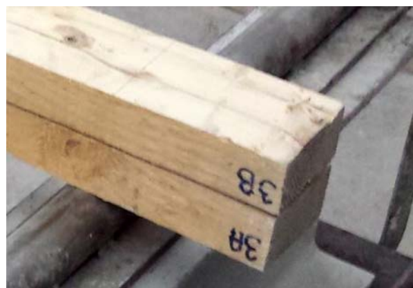
Fig. 15. Timber beams cut in half
