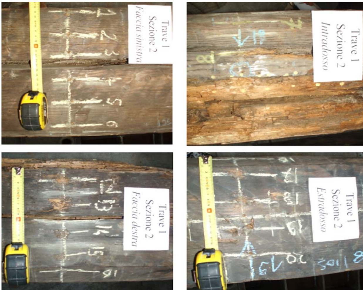
Fig. 4. Details of the beam 4 faces with tomography stations after data acquisition: left face and intrados (top left and right), right face and extrados (bottom left and right)
