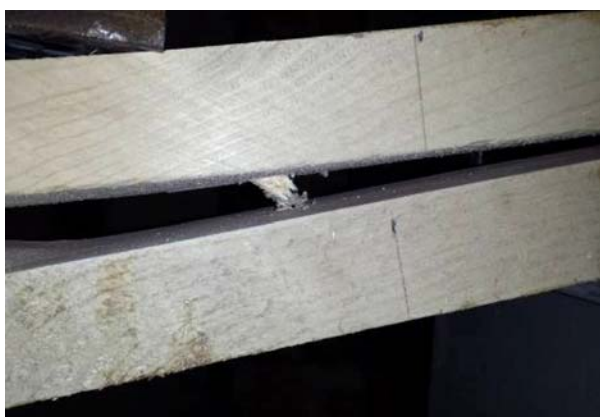
Fig. 17. Pull out of the BFRP spike
