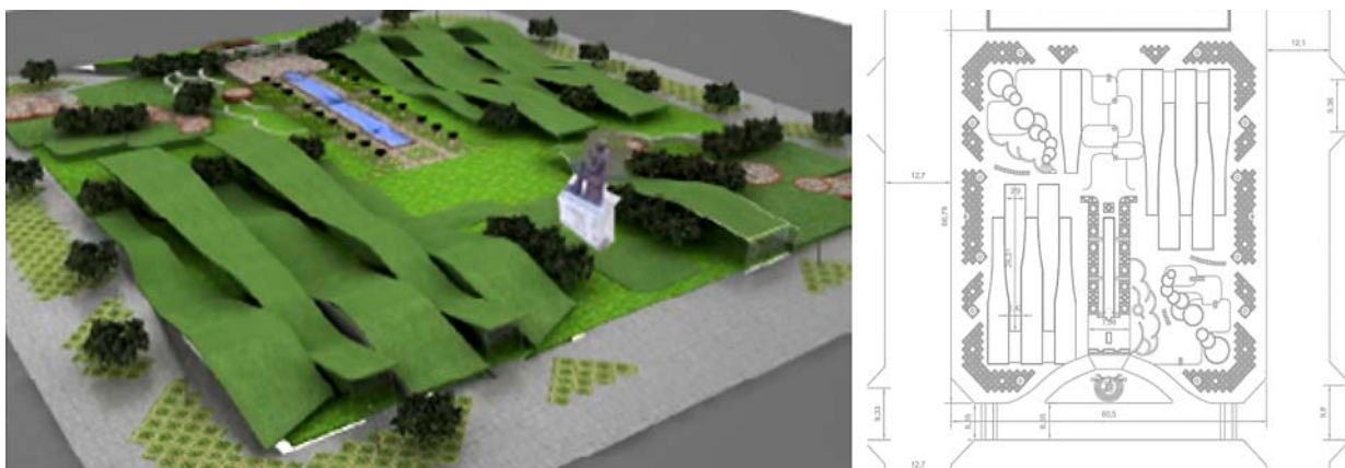
Fig. 6. Showing 3D model of the parking lot green roof in the park drawn in the left photo
