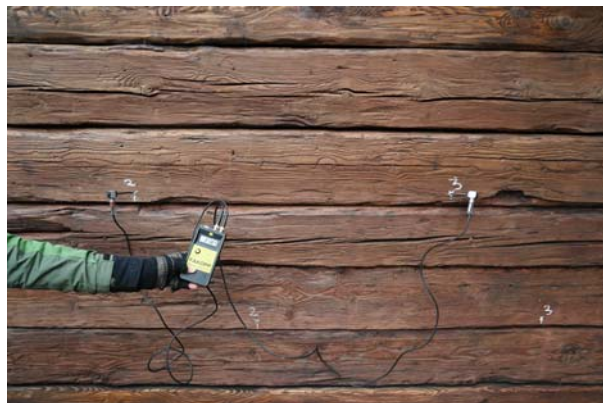
Ryc. 10. Urządzenie Fakopp Microsecond Timer podczas pomiaru Fig. 10. Fakopp Microsecond Timer device during testing
